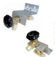
ME-1 contains inlet connection with shut-off valve, non return valve, collecting pipe and two outlets. Bodies of components are made of brass. Stabile wall bracket made of 3mm stainless steel is used as a base for components mounting. ME-1 is prepared for 300 bar service.
