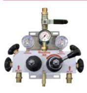
Single-stage semiautomatic autochange gas manifold for compressed gases with inlet pressure up to 300bar. This product can ensure continuous gas supply without any application process interruption. Manifold can be equipped as an option by contact gauges to give information about gas source emptying. Product consists of massive brass block which is the stabile base for other components installation.
