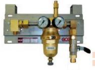
New concept of gas manifold with similar features as MU70-M. O, D, N,  $CO_2$  variant is equipped by high-flow regulator MR400. Manifold unit with mounted hanging kit is shown at the picture. Hanging kit contains two stainless steel hangers, screws with nuts and washers and also two outlet adaptors with threads G1/4" and G3/8" for direct hose installation. This kit can be used in combination with MU70-M or MU400-M manifolds.
