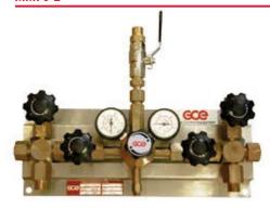
Manual changeover manifold for different gases with inlet pressure up to 300bar. At both inlet sides is placed x-block with non return valves and filters, purge valves and second inlets from sites for extension units. Shut-off valves, regulator with pressure relieve valve and outlet ball valve as well as other components are mounted at the stainless steel panel.
